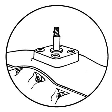
the factory and should not be adjusted unless it is desirable to operate the pump above the minimum volume. This is done by loosening the lock nut and turning the adjustment nut clockwise until the minimum flow desired is reached, then tighten lock nut.
