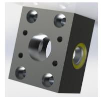
Aluminum inlet block with Port size reduction from 3" split flange to 2" split flange and two 1" SAE ORB port to accept the returned flow from the unloading blocks. It eliminates the need for a large inlet hose from the reservoir.
